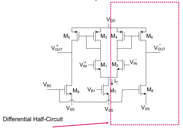
Note: Source node of M<sub>1</sub> and M<sub>2</sub> at ac ground with differential excitations
