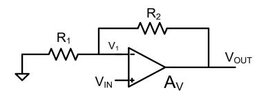
$$A_{VF} = \frac{V_{OUT}}{V_{IN}} = \frac{1 + \frac{R_2}{R_1}}{1 + \frac{1}{A_V} \left(1 + \frac{R_2}{R_1}\right)}$$
