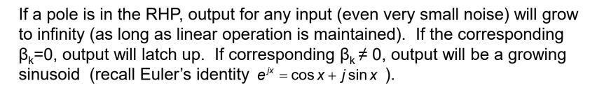
Theorem: A linear system is stable iff all poles lie in the open left half-plane
